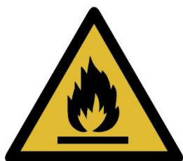
Caution, risk of fire R290
